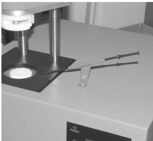
RVA showing syringe for adding NaCl to the RVA can.
